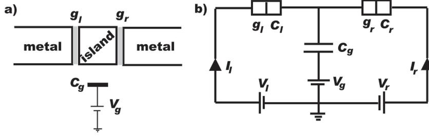
FIGURE 1. a) Sketch of the SET device. b) Equivalent circuit of the SET.
