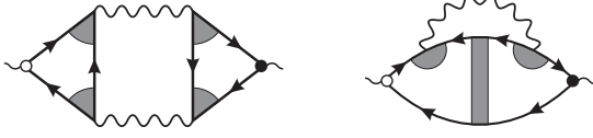
FIGURE 1. The Aslamazov-Larkin (AL) and density-of-states (DOS) diagrams for the thermoelectric response \tilde{\beta}^{xy} . The DOS diagram has a symmetric counterpart. The white and black circles correspond to the different heat and electric vertices, the shadowed blocks represent cooperons, and the wavy lines denote the fluctuation propagator (see text). All objects on these graphs are generally matrices in the Landau basis.
